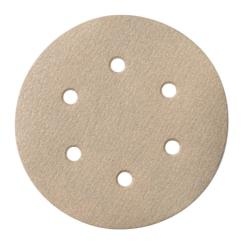
25 Hook and loop sanding sheets, 150 mm, P 60, "paint", "professional" series for paints, lacquers, and filler compounds, for random orbital sanders, aluminium oxide, stearate-coated
